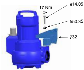
Fig. 10: Fastening the claw for single guide rail
